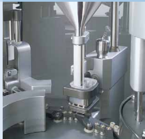
Each cycle renders performance: pellet filler with volumetrically adjustable filling volume.
