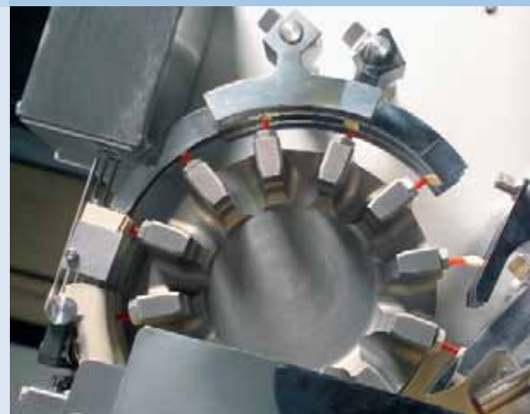
Piece by piece: No size constraints due to vacuum pick-up – the big plus of the tablet feed system.
