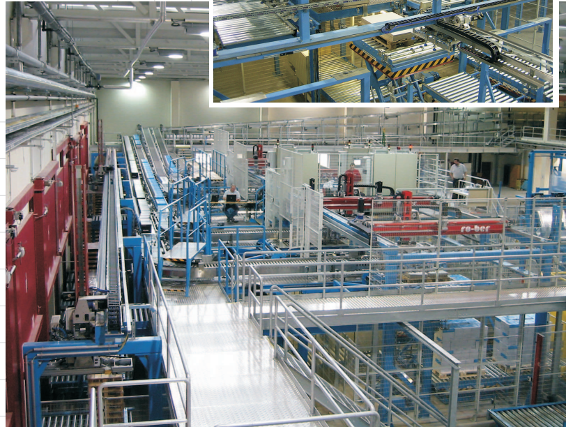
View of the palletising area with four palletising robots and a linear portal robot for empty pallet distribution
