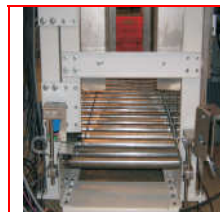
Stacker infeed with light curtain protection.
